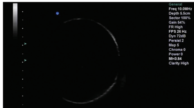
MP 4.4. Figure 3. Representative ultrasonographic image of water-filled balloon without evidence of CO 2 formation after sonication.
