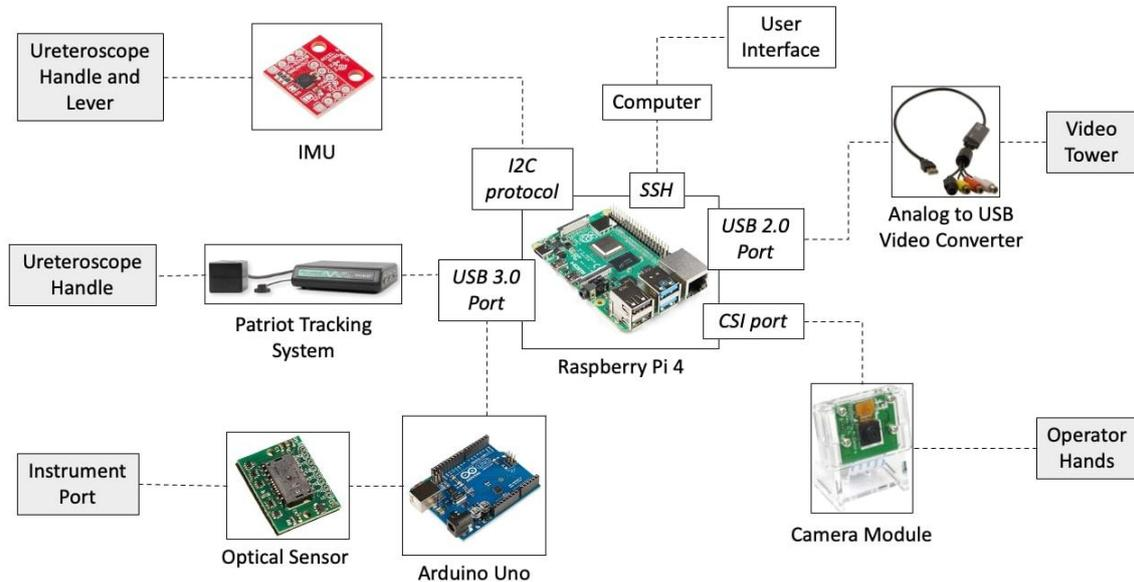
**Figure 2.** Complete motion-tracking and video-capture tool. A) B) Inertial measurement unit and Patriot standard sensor fitted onto the single-use flexible ureterorenoscope. C) Optical sensor fitted to project above the insertion point of the ureteroscope onto a simulator box. D) Complete view of tool with Patriot source (i.e., reference coordinates for x, y and z axes) and Raspberry Pi camera module pointing toward operator's hands.
