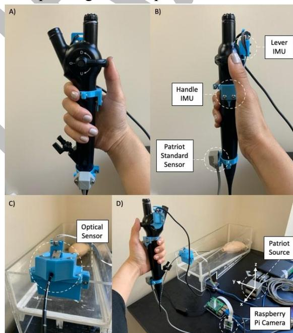
**Figure 3.** Illustration of the measurement of roll, pitch and yaw in relation to the rotational movement of the ureterscope, and translation at the insertion point.
