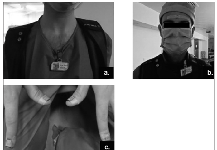
Fig. 2. Dosimeter position representation (a) Radiophotoluminescence (RPL) dosimeter on torso under lead apron; (b) RPL on neck and thermoluminescent dosimeters (TLD) for lens; (c) TLD on extremities.
