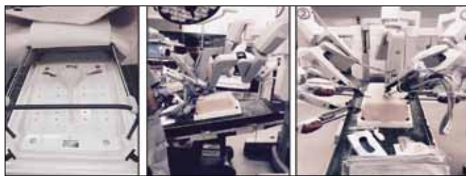
Fig. 1. Setup of 3D printed bladder model within the realistic pelvic silicone torso.
