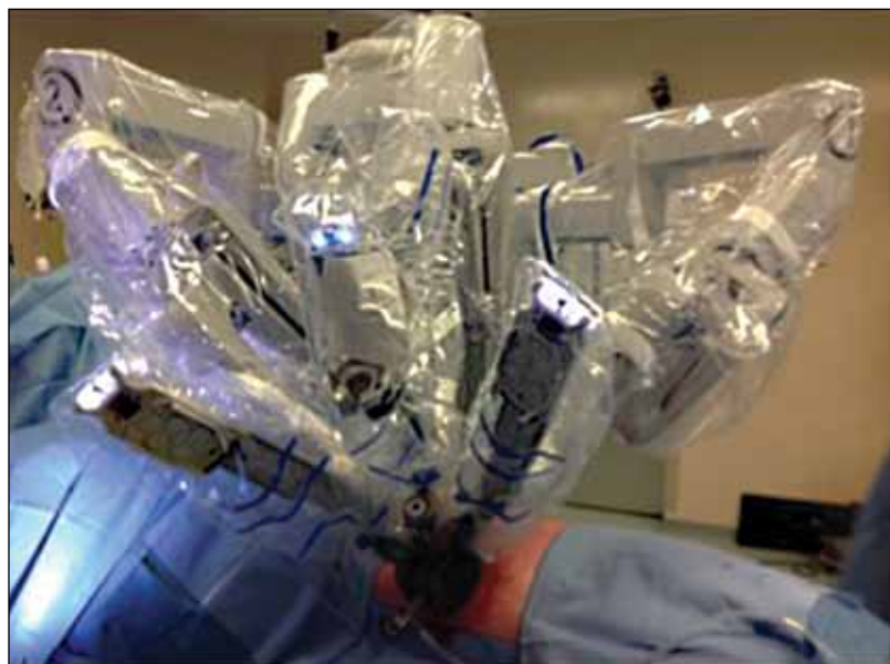
Fig. 1. (A) Positioning of the robot over the posterior shoulder of the patient for single-incision surgery. The patient is positioned at 45 degrees in the right lateral oblique position; (B) The first setup joint is locked in a straight position to facilitate proper insertion of multiple working instruments in the umbilical port. Rendering © Intuitive Surgical 2015 with permission.
