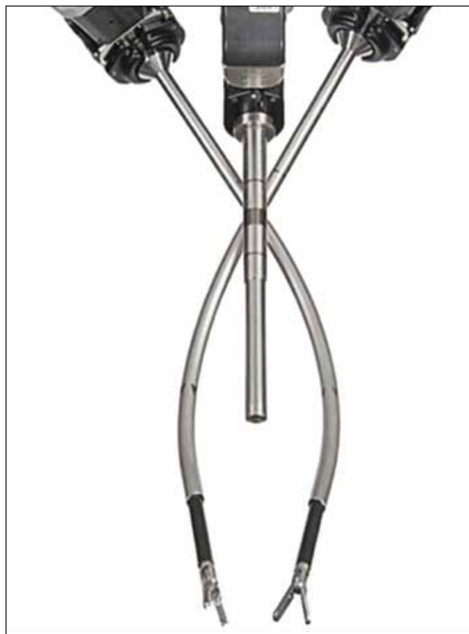
Fig. 5B. Image of the single-site (Intuitive) ports and instruments. The instruments cross at the level the fascia. The curved ports and flexible instruments provide separation between instruments and the camera. However, dexterity is limited by the lack of wristed instruments for the current platform. Rendering © Intuitive Surgical 2015 with permission.
