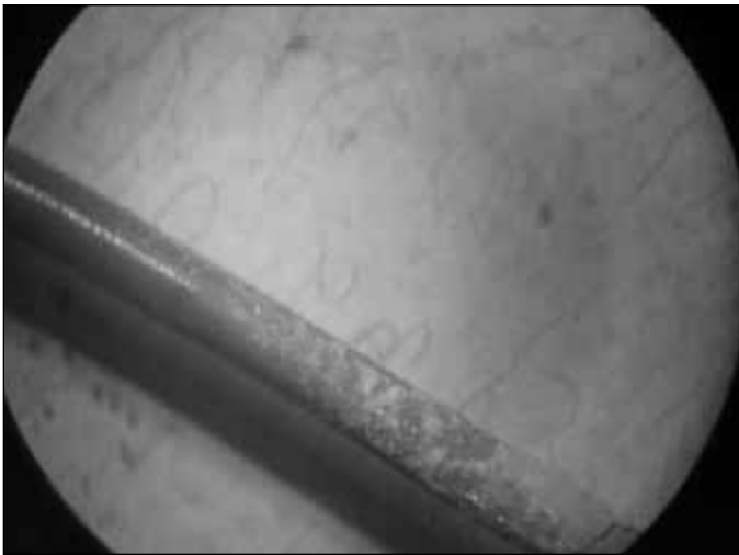
Fig. 9. Removed polyurethane ureteral stent fragments were noted moderately encrusted and breakage lines are noted along the stent side hole.
