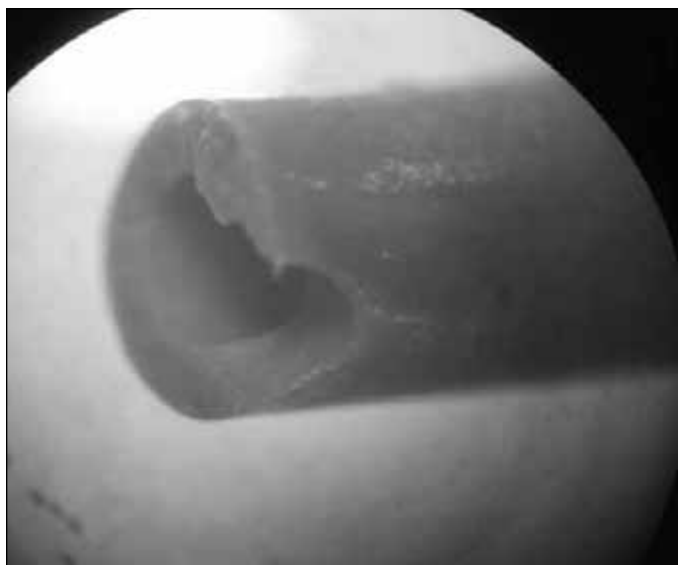
Fig. 7. Second image: microscopic imaging of the stent fragment (magnification \times 500 ) showing line of breakage traversing the polyurethane ureteral stent side hole near the distal bladder end.
