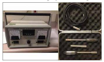
Fig. 1. Electroejaculation machine and probes.
